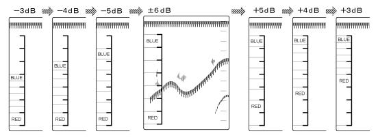
This picture shows the comparative signal threshold levels to the standard ±6dB for the dynamic ranges.
