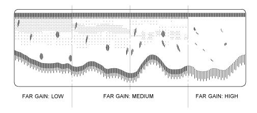
Selecting STC function releases the gain adjustment automatically so that the sensitivity of the receiver becomes weaker in the distance.
